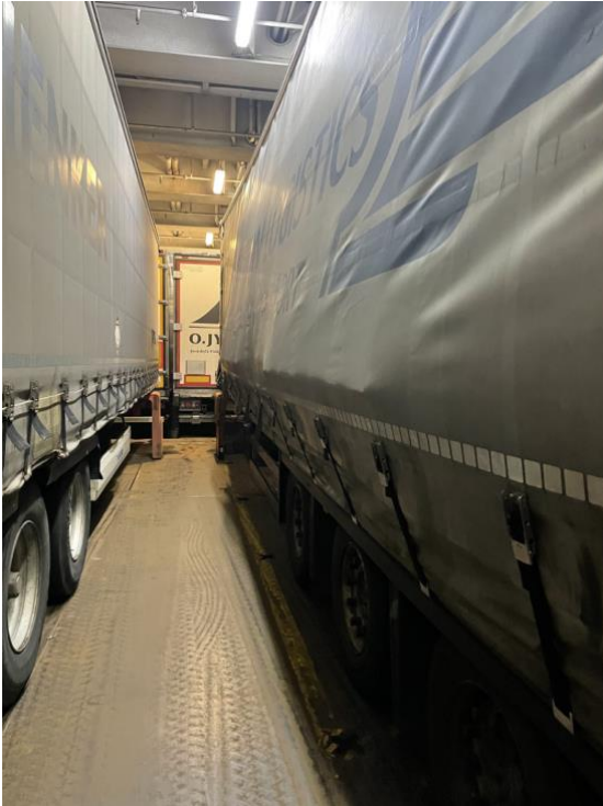
Figure 26: Inadequate lashings inside the unit.
