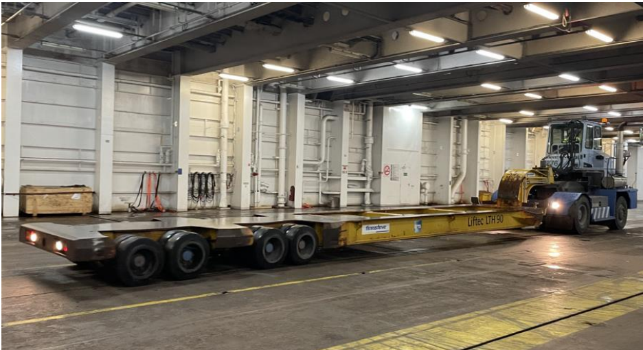
Figure 4: Rolux system connected to a terminal tractor. Rolux is used for stowing cassettes.
