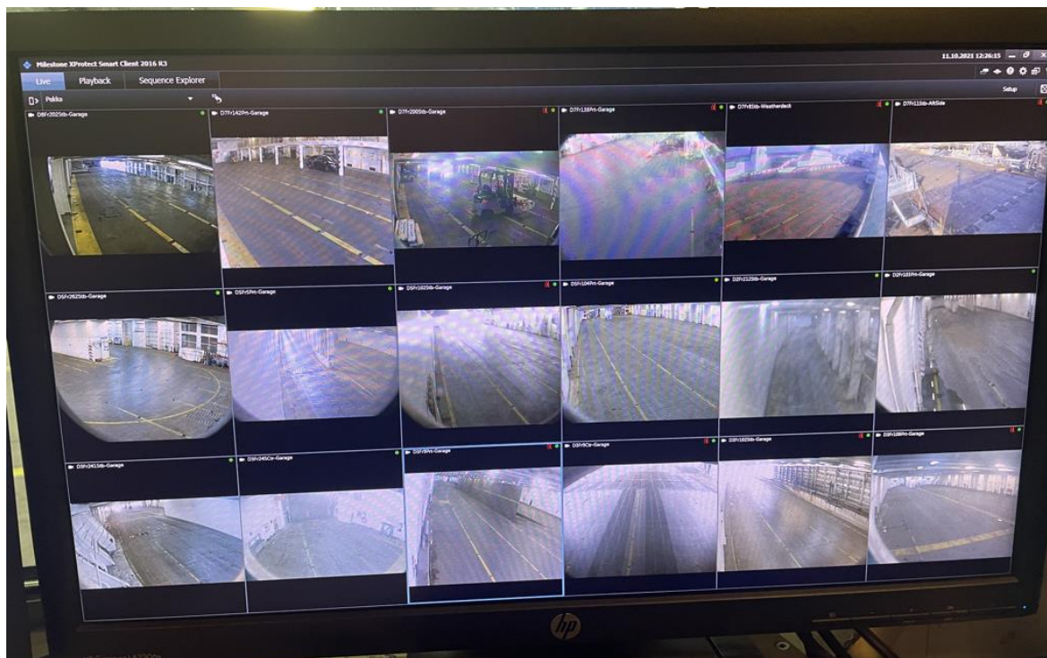
Figure 19: CCTV helps Chief Officer to follow real time situation of the loading.
