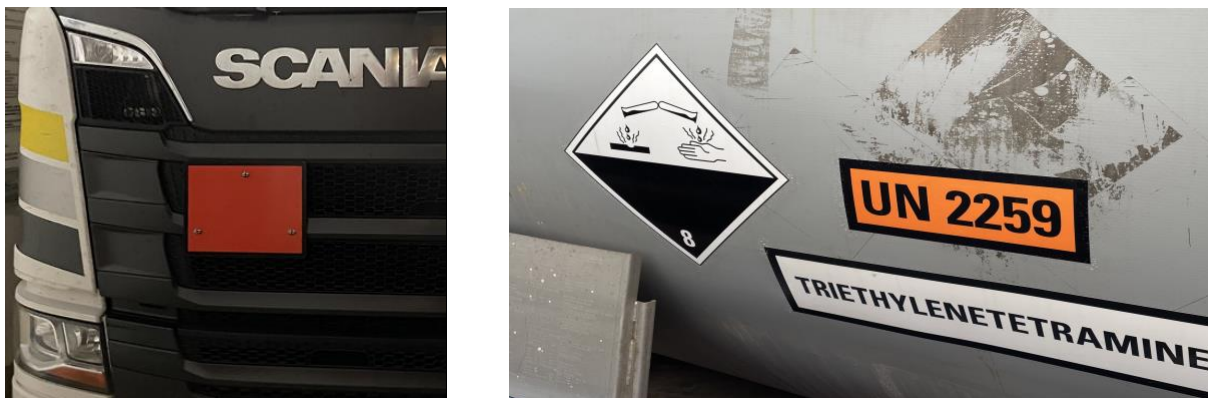
Figure 12: Orange placard informs that the truck is carrying IMDG cargo in a packed form.
