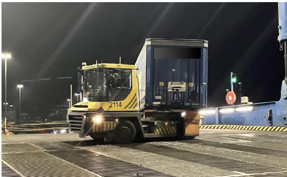
Figure 9: Terminal tractor loading a semi-trailer onboard.
