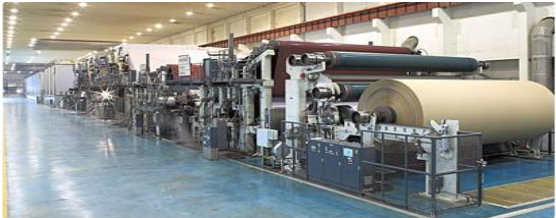
FIGURE 2. Board making by a Metso-supplied machine in China. (Changle Numat PM1: a benchmark for producing white top liner in China 2012.)
