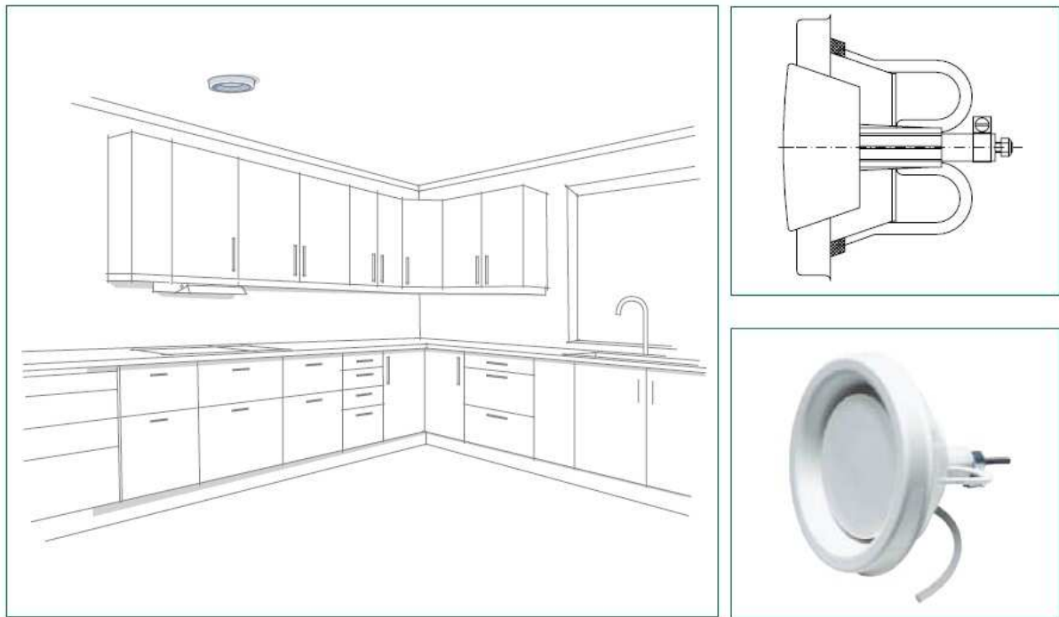
FIGURE 10. Control exhaust valve KSOM with humidity sensor/14/
