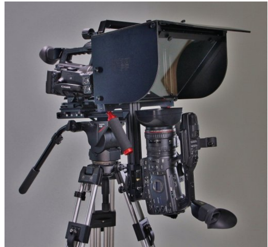
Filmfactory's Mirror rig aka beamsplitter rig. 5
