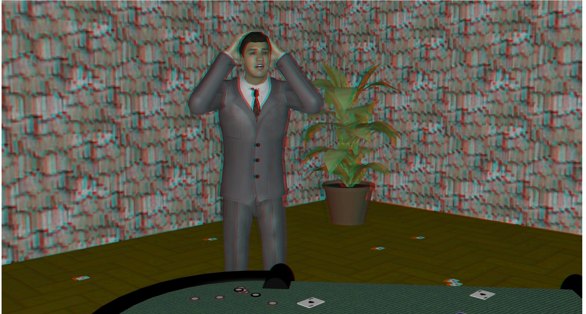
SMALL INTERAXIAL WITH OBJECTS FARTHER. With a very small interaxial of 29mm this image produces quite disapointing 3D effect. The closest object at 0% and far parallax 1%
