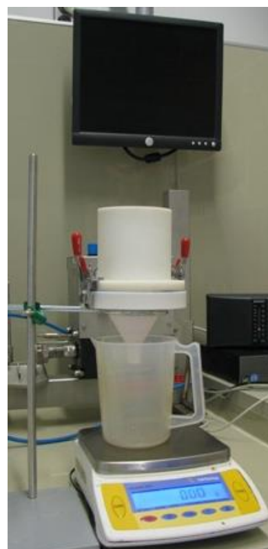
FIGURE 12. Gravity filtration measuring set-up. Photo taken by Kaisa Kätkä.
