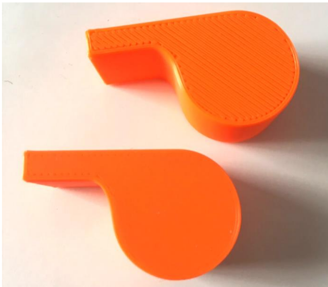
Figure 6. First layer configured well (below) and nozzle too high (above)
