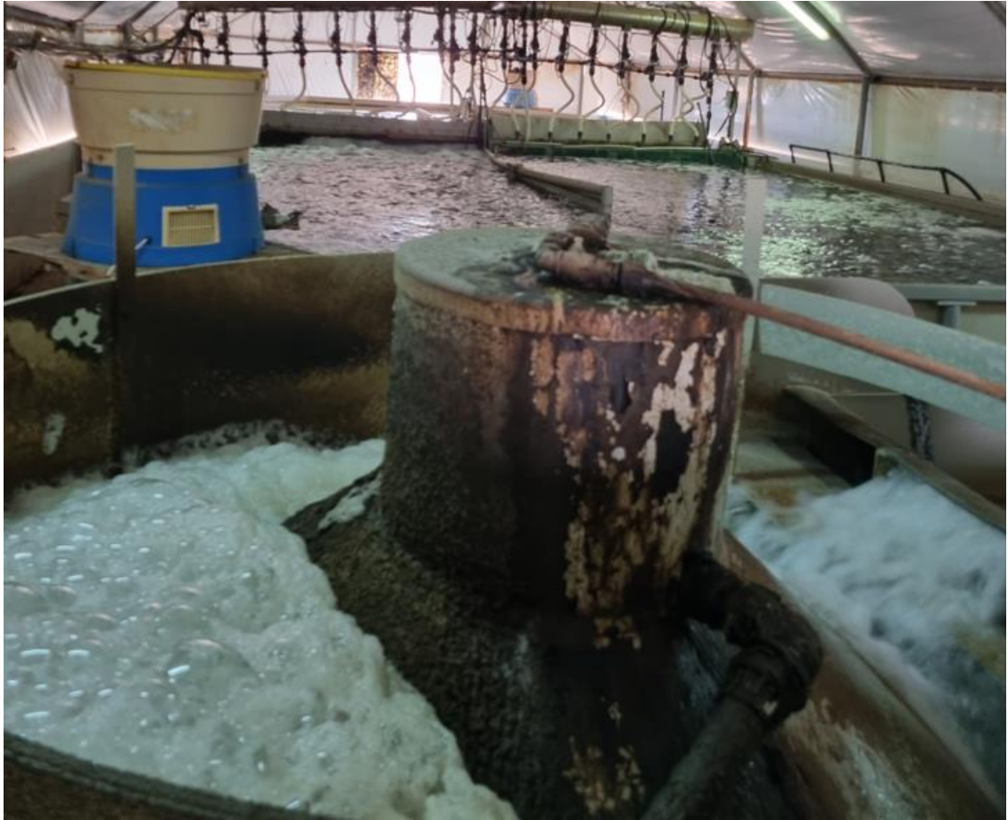
PICTURE 1. Foaming protein skimmer in RAS (Yogev 2022)
