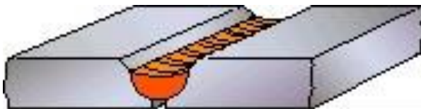
Pictures 12 incomplete root penetration [4]
