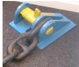
Figure 12 & 13. Pins with red top and shark jaws in red, roller in yellow
