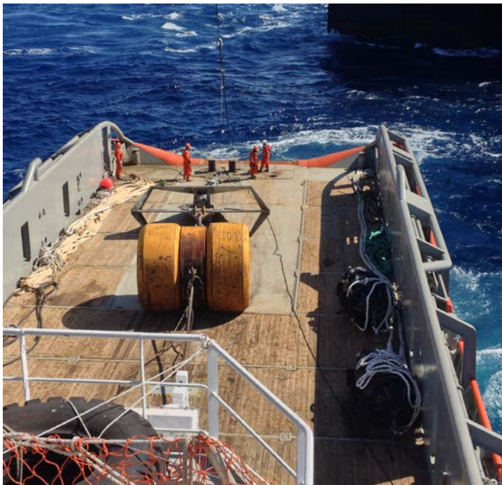
Figure 24. AHT Preparing for anchor run
