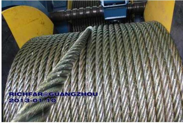
Figure 4. Commonly used 64 mm tow-wire
