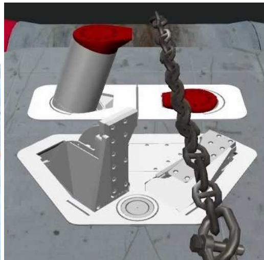
Figure 12 & 13. Pins with red top and shark jaws in red, roller in yellow
