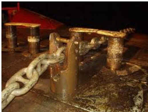
Figure 14. Karm Fork and Pins
