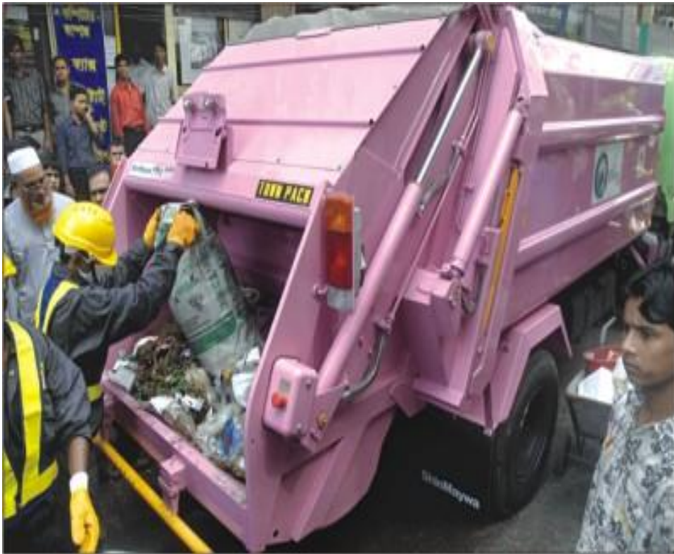
Figure 13: Using compactor trucks to collect wastes from community dust bin and secondary container in Dhaka city. (DCC)
