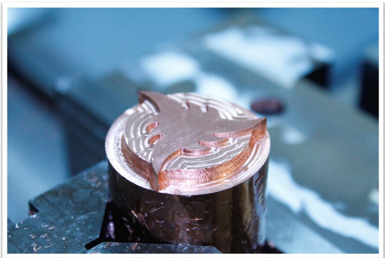
Figure 21: Electrode milled in Arcada's lab.
