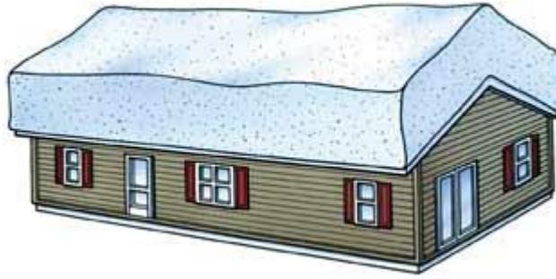
Figure 14 Snow load accumulated on a building (North roof load zone, n.d.)
