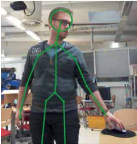
Figure 8. Kinect application recognises the user lifting his left arm and turns the lights off.
