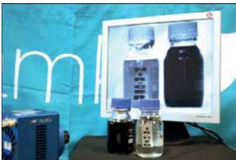
Figure 6. Near infrared imaging used in moisture detection and in seeing through kerosene based liquid.
