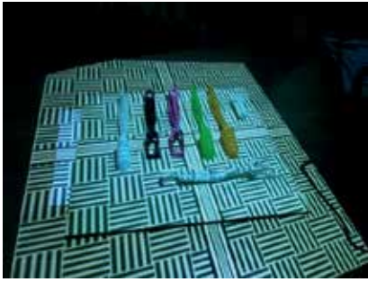
Figure 2. Fringe lighting pattern on the target.
