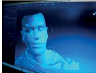
Figure 3. 3D model of a human made with fringe based scanning imaging system.
