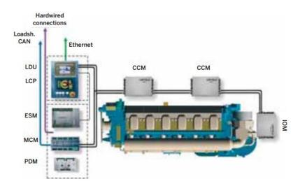
Figure 4. UNIC Bus design and main components. [3]
