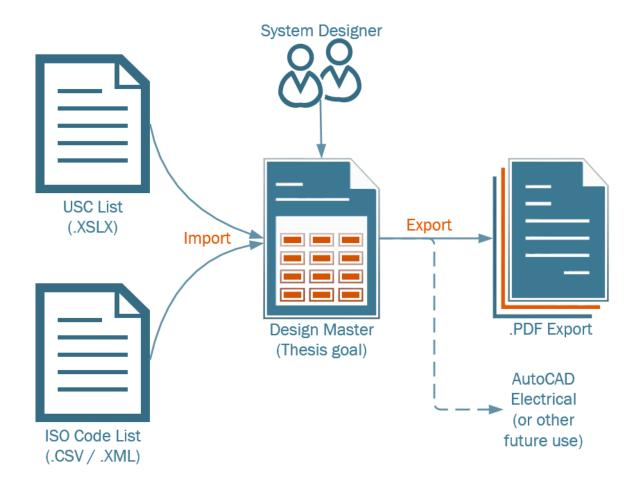
Figure 2. Data flow visualized. Design Master template semi-automatically updates data sources (USC and ISO) with VBA. It can also export the completed design as a .PDF file
