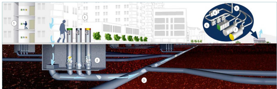
Figure 3. Pipeline-based waste collection system, stationary system (Envac, 2008)
