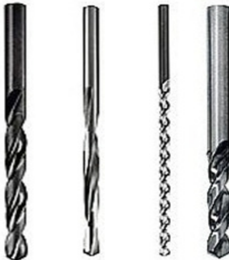
Figure 7. Starting from right, stubb drill, long series drill, jobber drill, standard drill
