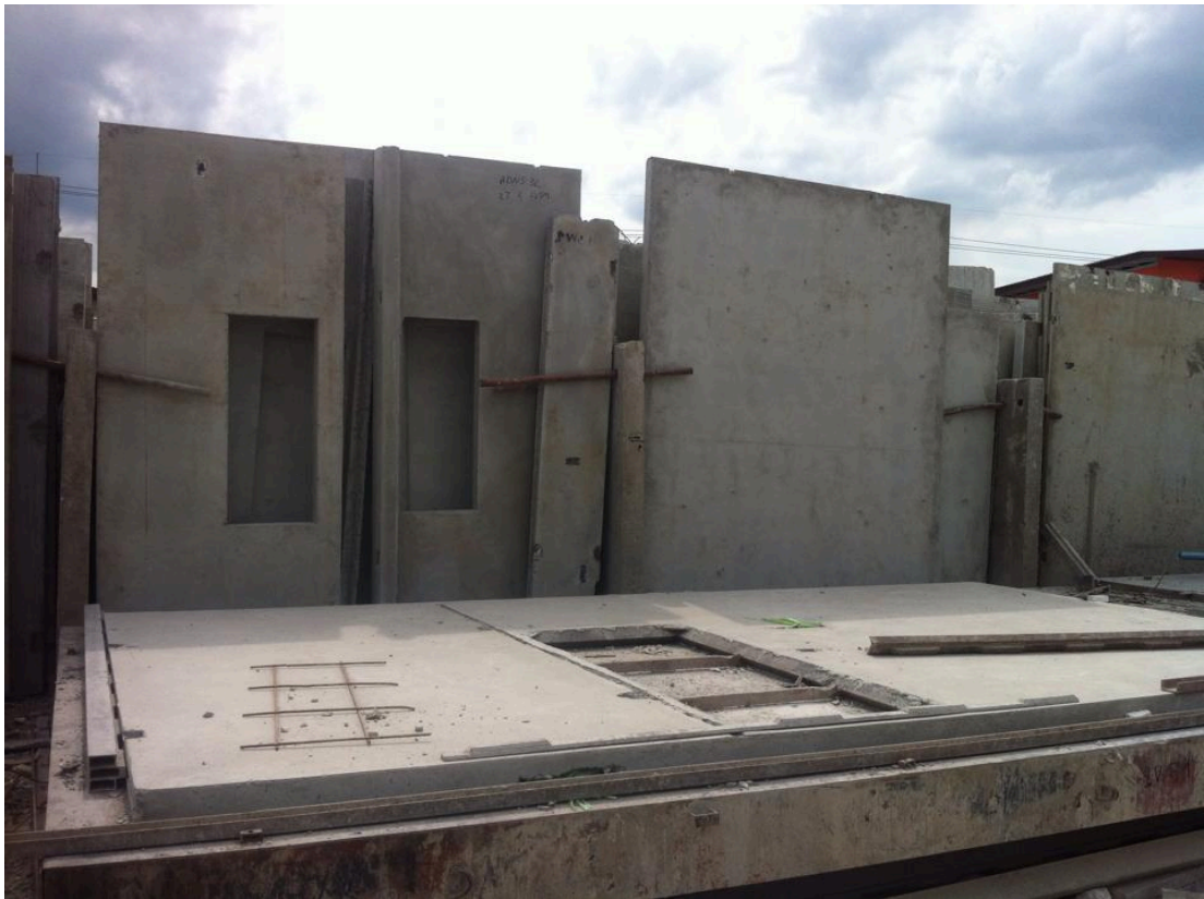
IMAGE 11. Precast wall elements in the Pro-Build precast concrete factory
