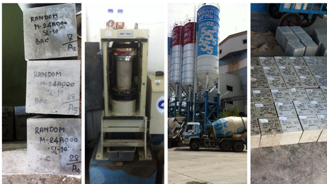
IMAGE 7. Cubic concrete test samples and compressive strength testing in the CPAC concrete factory (Kuronen and Turunen 2014-05-28).
