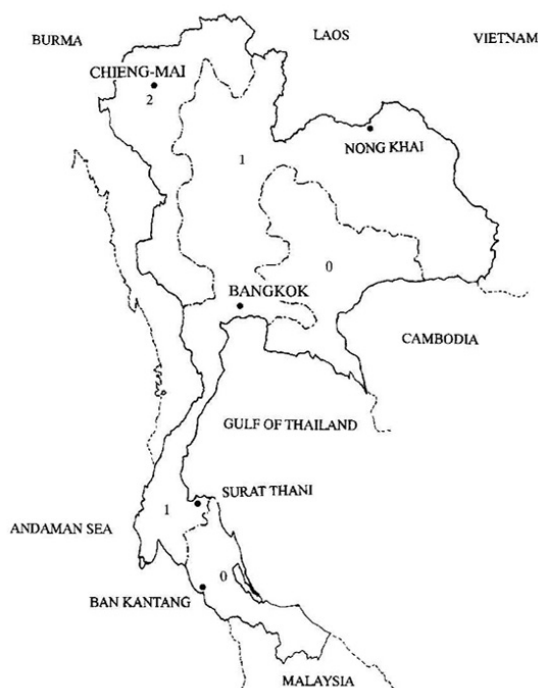
FIGURE 2. The map shows where seismic activity has to be taken into account when planning the structures (International Institute of Seismology and Earthquake Engineering 2000-2003)
