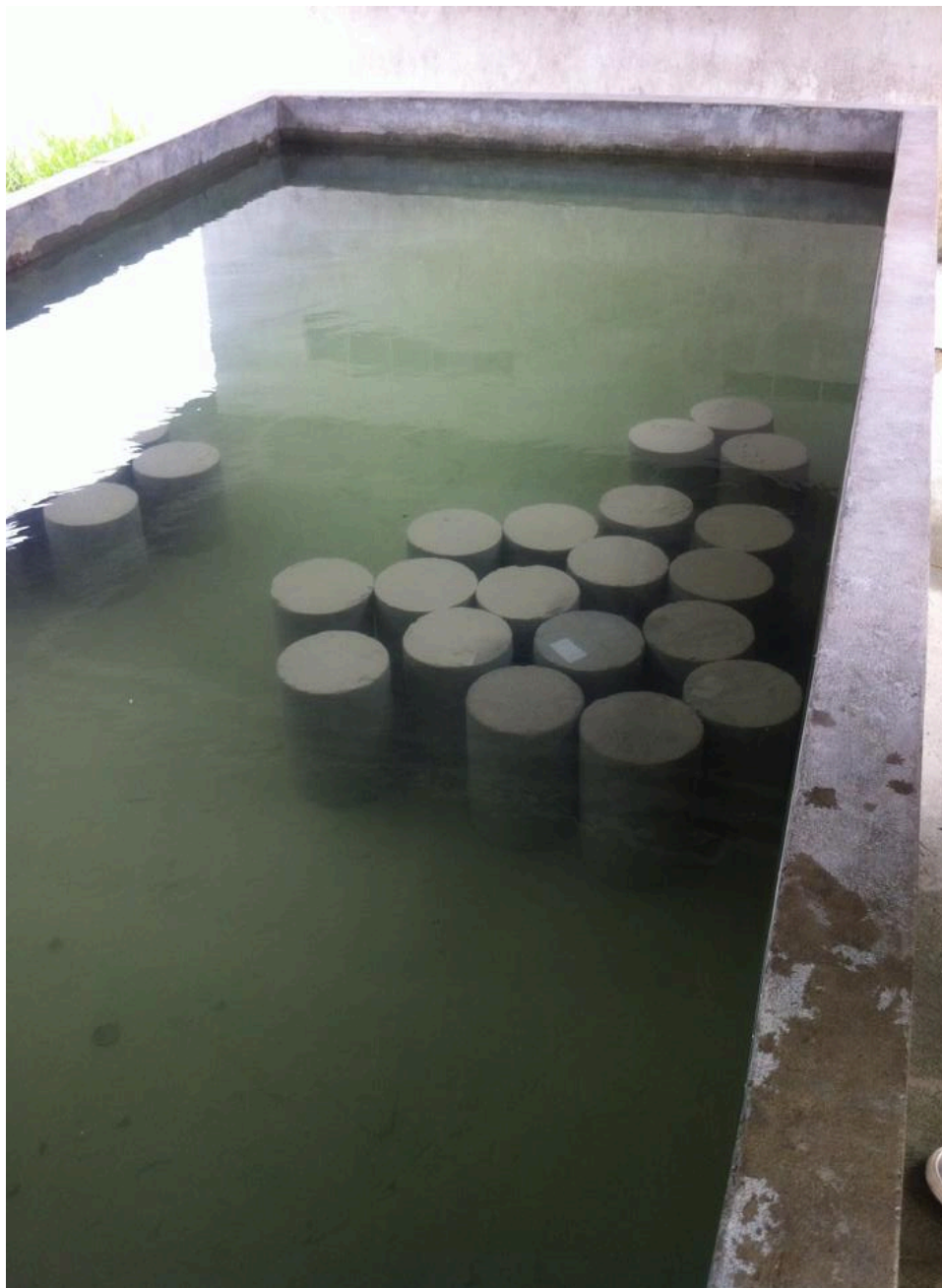
IMAGE 6. Cylinder concrete test samples in CPAC concrete factory (Kuronen and Turunen 2014-05-28).
