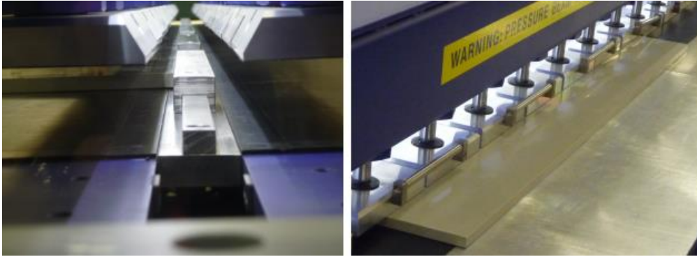
Figure 13: Alignment of the Sheets (Left). Clamping the Sheets (Right) (Picture by Author)
