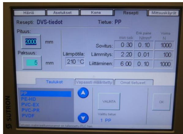
Figure 12: Machine's Display showing the Corresponding Welding Force, Tool Temperature and Duration for the Inserted Parameters (Picture by Author)
