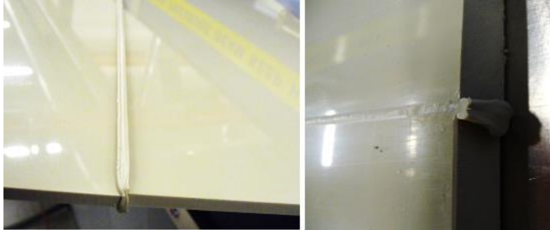
Figure 16: Sheet before Bead Removal (Left). Sheet after Bead Removal (Right) (Picture by Author)
