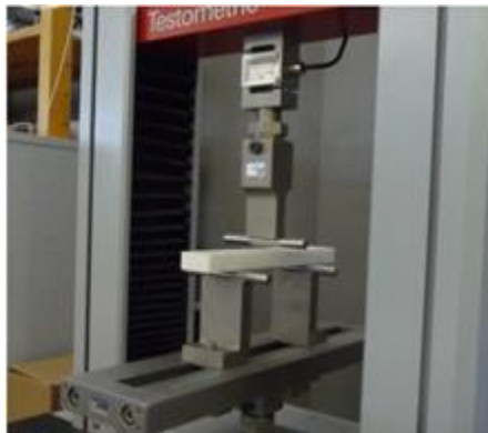
Figure 18: Bending Test Setup (Picture by Author)
