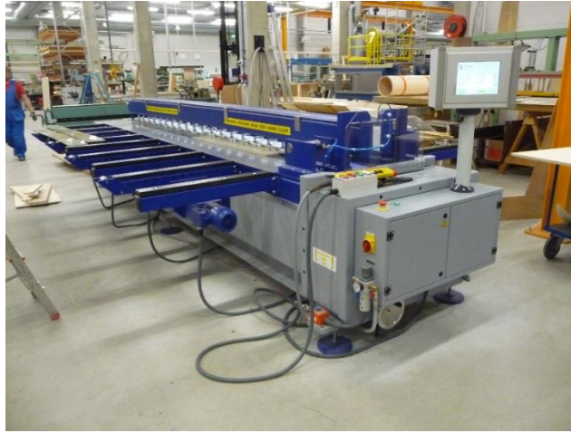
Figure 9: Sheet Butt Welding Machine Wegener SM 440 TPQ (Picture by Author)
