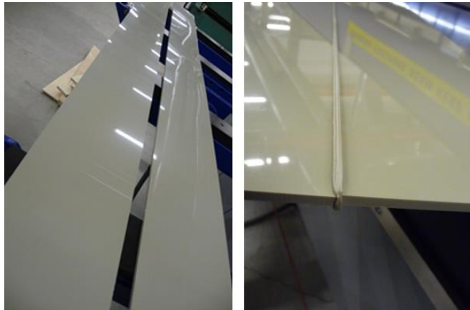
Figure 11: PP Sheets Before and After Welding (Picture by Author)
