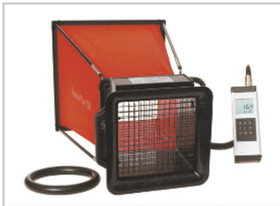
FIGURE 16.SWEMA air 300 flow device with sensor “Swema flow 125” /16./
