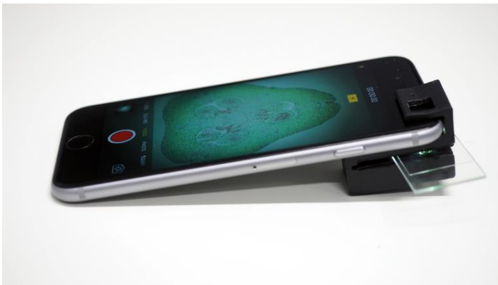
Figure 7: A 3D-printed clip-on attached to a smartphone. (England, 2018)
