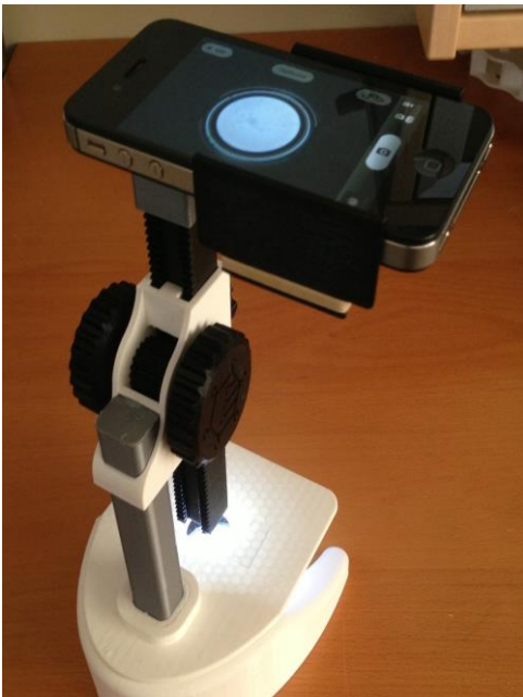
Figure 8: A 3D-printed platform for phone attachment. (Kwalus, 2013).
