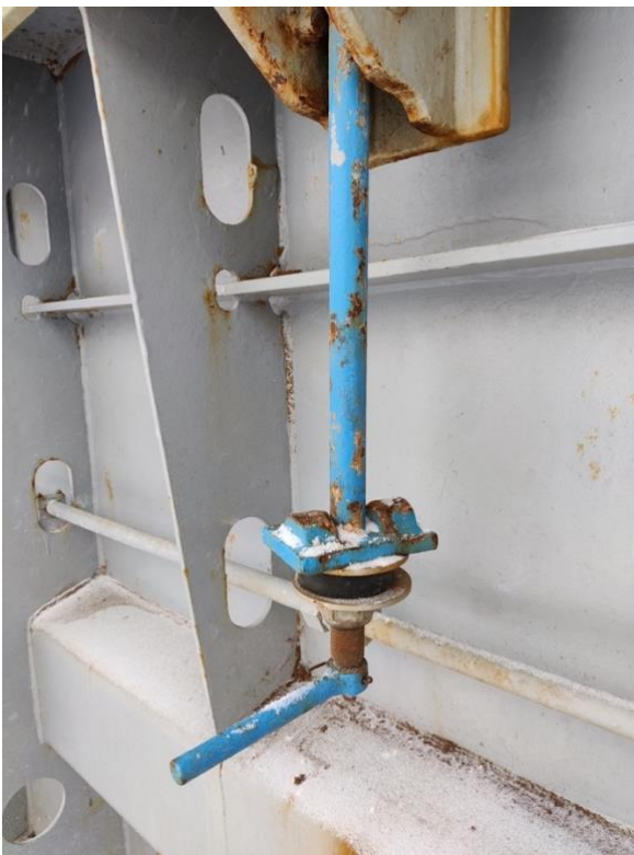
Figure 35 Quick acting cleat open position. (Matti Heinonen 2021)
