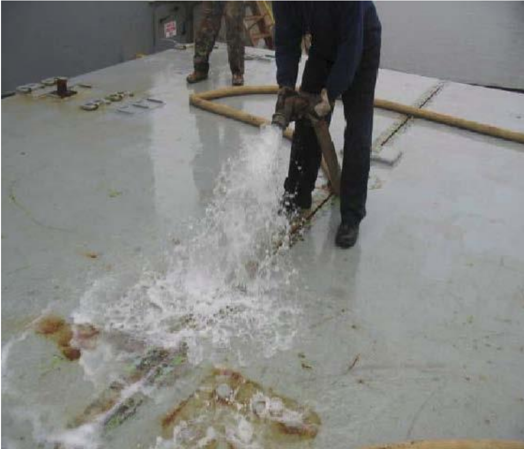
Figure 8 Hose testing (Bulk Carrier Guide, 2010)
