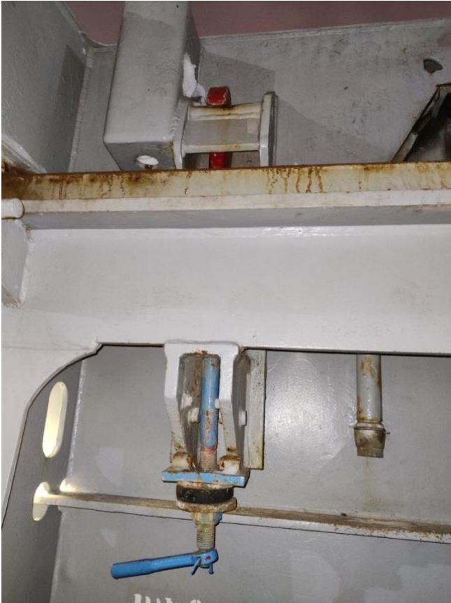
Figure 36 Quick acting cleat closed position. (Matti Heinonen 2021)
