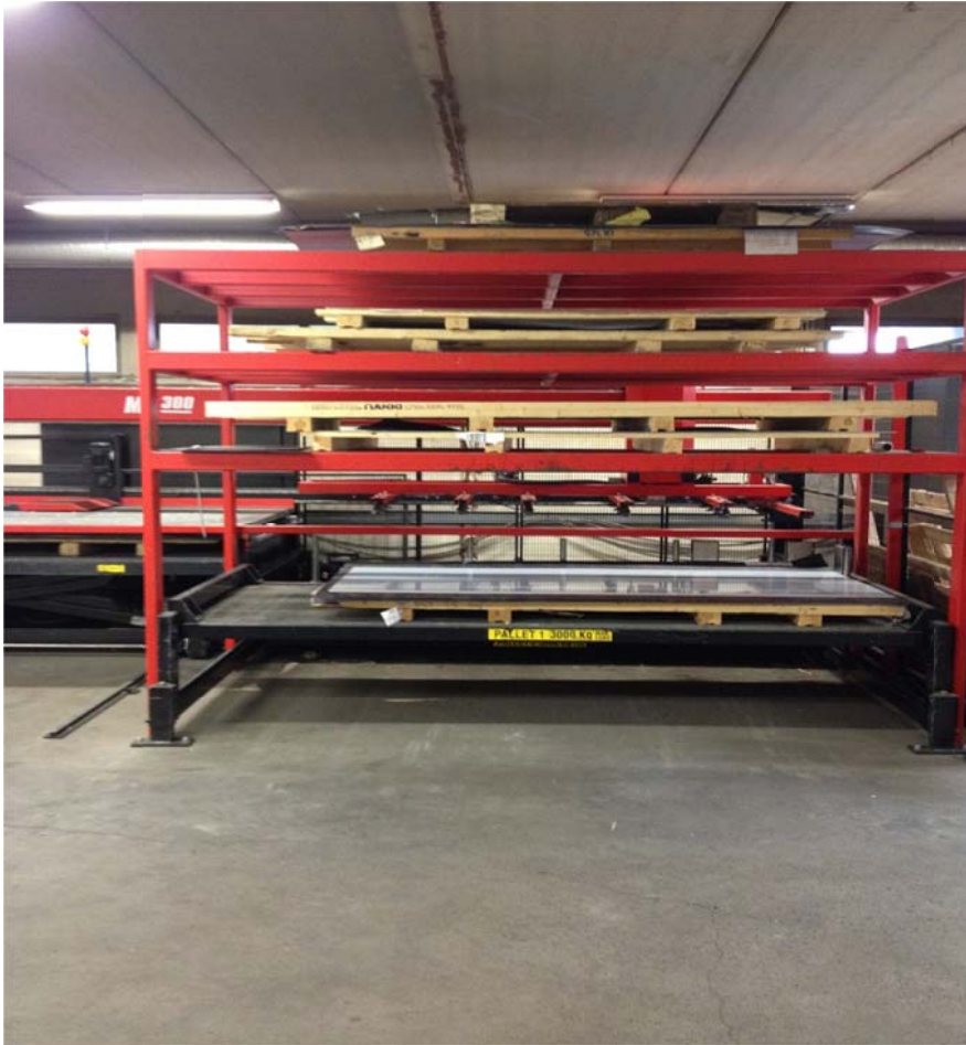
Figure 18 Sheet storage shelf improvement idea. Picture by Minna Kiuru August 2012.
