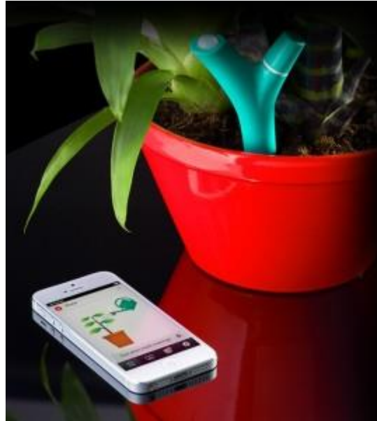
FIGURE 13. Plant monitoring application running on the mobile, communication with sensor
