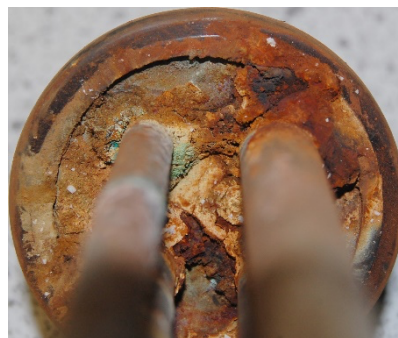
PICTURE 7. Aqueous corrosion (LPD Lab Service)
