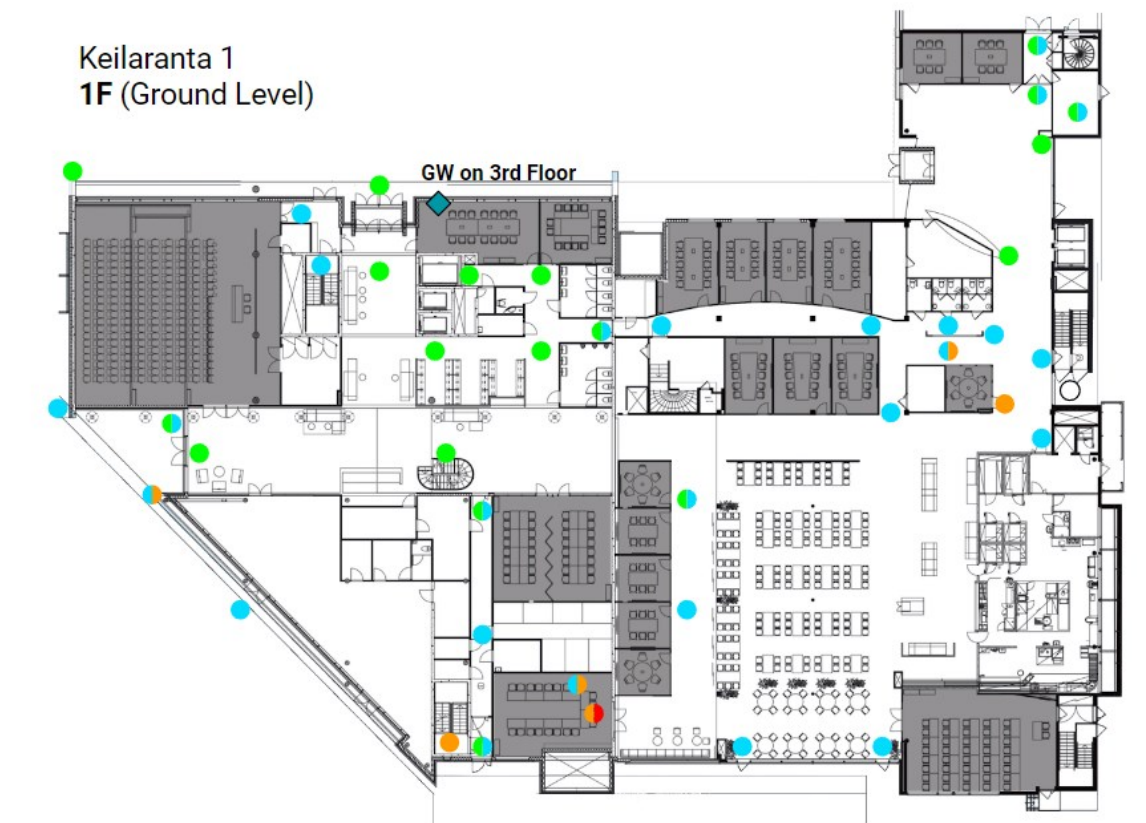
Figure 38. Anchor to Gateway communication range test.
