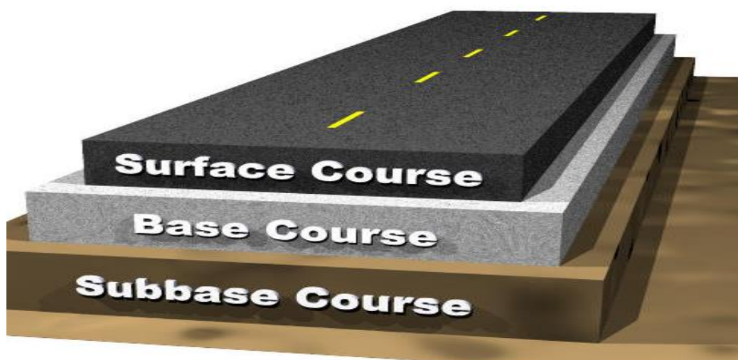
Figure 9. A practical view of a road pavement construction.
