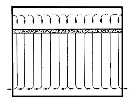
Figure 6. Unidirectional downflow air distribution. /7/
