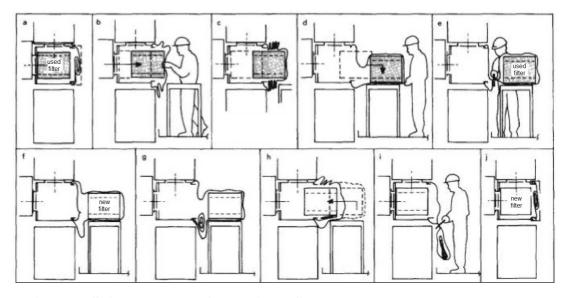
Figure 8. Safe procedure of changing a filter. /7/
