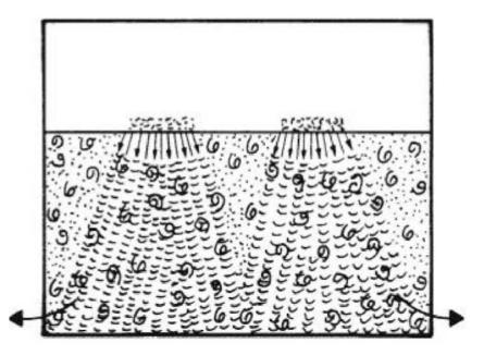
Figure 5. Turbulent flow air distribution. /7/
