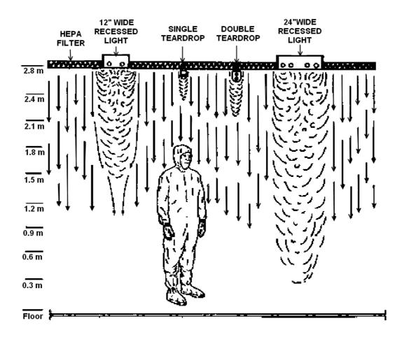
Figure 7. Obstruction cased turbulence in a laminar flow cleanroom. /7/
