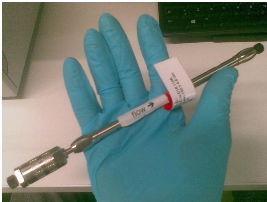
Figure 6. Phenomenex Gemini-NX 5µm C18 110A column with a guard column attached.
