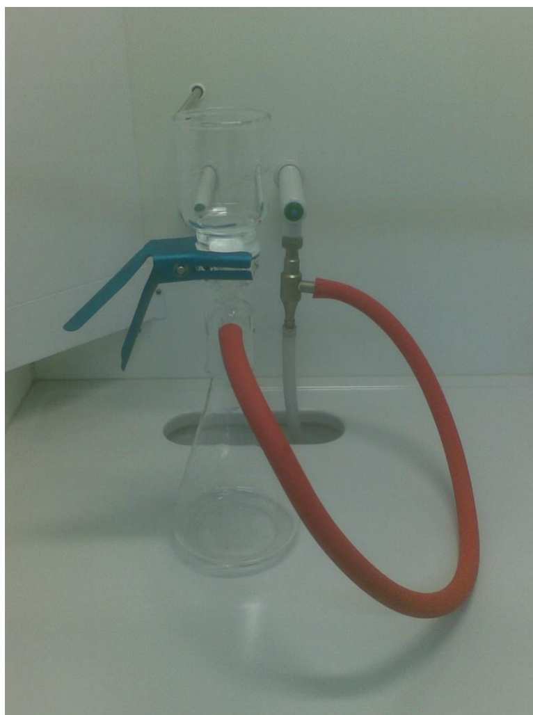
Figure 8. Vacuum filtration unit used for preparing eluent A.
