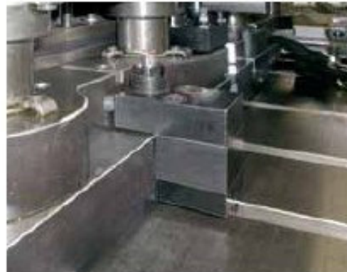
Mechanical sliding clamps fastened to a machine bed.
